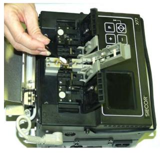
• Use a Coventry 6704 Lint Free Wipe with ITW Chemtronics CP410 for cleaning of key pads and other surfaces. ITW Chemtronics CP400 is a high quality IPA solvent source for cleaning mirrors.
